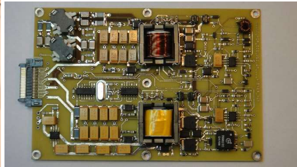
Figure 2. Engineering model of power supply unit supporting 2 DPUs and 3 sensors and individual power supply unit of JDC sensor (Jovian plasma Dynamics and Composition)
