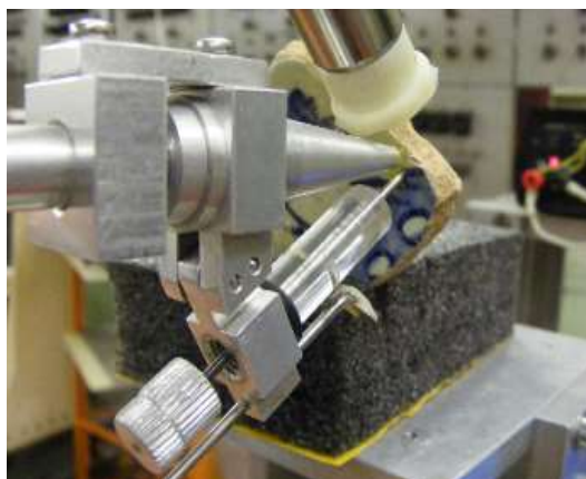
Figure 2. PIXE analysis of a dark blue area on Iznik glazed ceramics sherd (sample: CER 9)
