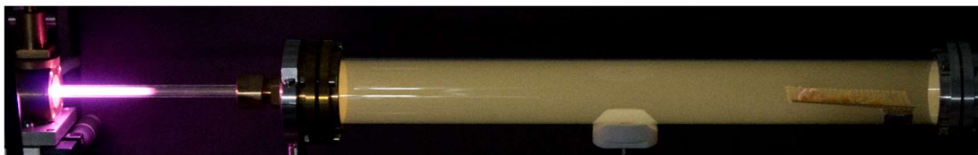
Figure 3. The post-discharge system with the surface-wave microwave discharge operating in N 2 -20%O 2 mixture during seed treatments.
