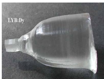
Figure 1. High optical quality LYB crystal doped with Dy.
